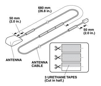
27. Wrap five of the cut pieces of urethane tape around the antenna cable at the measurements shown.
