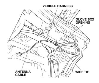
36. Route the antenna cable through the glove box opening and toward the center panel.
