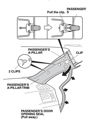
• To prevent clips from falling into the body panel area, carefully insert a shop towel between the passenger's A-pillar and the passenger's A-pillar trim.
