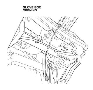
35. Using one wire tie, secure the antenna cable to the vehicle harness.
