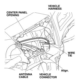
38. Using one wire tie, secure the antenna cable to the vehicle harness inside the center panel.
