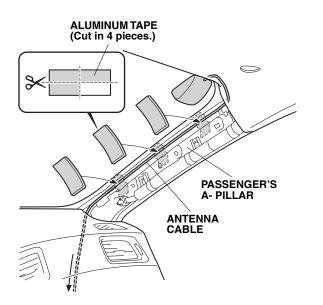
33. Route the antenna cable along the passenger's A- pillar. Using isopropyl alcohol on shop towel, clean the A-pillar where the aluminum tape will attach. Using three pieces of aluminum tape, secure the antenna cable to the A-pillar in the areas shown. NOTE: Be careful not to attach the aluminum tape over the holes in the A-pillar. 34. Route the antenna cable down behind the dashboard.
