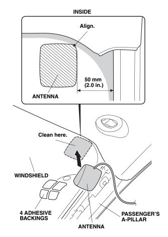
29. Remove the four adhesive backings from the antenna, and attach the antenna to the windshield at the measurement shown. Apply firm pressure to the antenna for at least 30 seconds.
