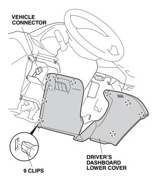
13. Remove the driver's inner dashboard trim (four clips and unplug the vehicle connector).
