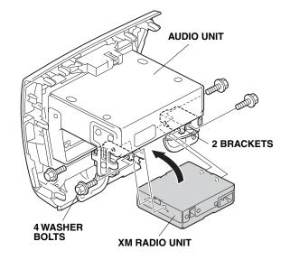
21. Tighten the two washer bolts installed in step 19.
