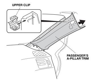
5. Remove the remaining upper clip from the passenger's A-pillar.
